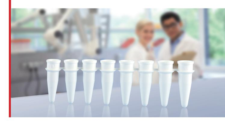
White tubes enable maximum fluorescence reflection in qPCR. Comparing to transparent products, 10-fold fluorescence levels can generally be measured with white disposables.
